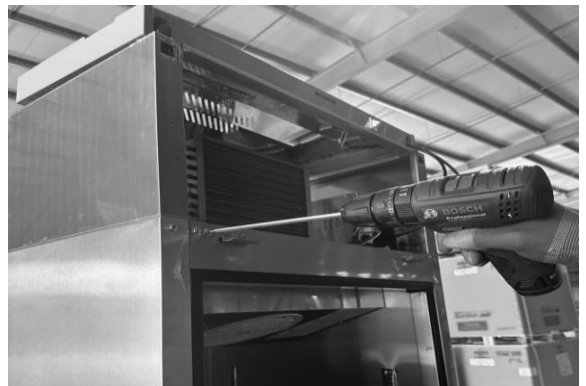
D-2. Unscrew screws located on top
