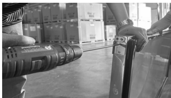
F. Disassemble the stopper plate, then tight screws
