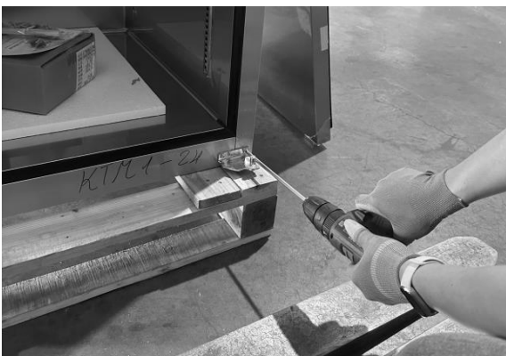
C. Disassemble bottom hinge
