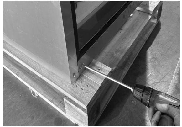
D-1. Unscrew screws located at the bottom
