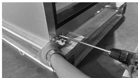
E. Assemble the bottom hinge
