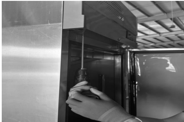
A. Disassemble the grille
