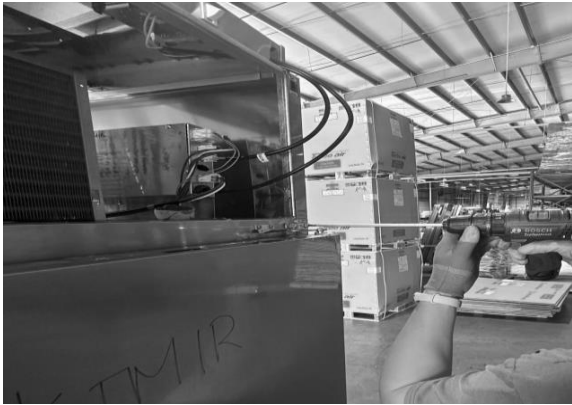
A. Unscrew screws located on top
