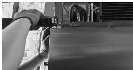
I. Assemble the hinge, then place the hinge into the hole on the inside
